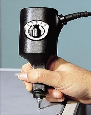
Marks can be engraved by use of a diamond-tipped pen, other sharp pointed tools or by the use of an electric engraver. A stencil is often used to ensure neatness when the mark can only be placed in an obvious position. Stencils also allow relatively small lettering which is not always the case when performing freehand.
